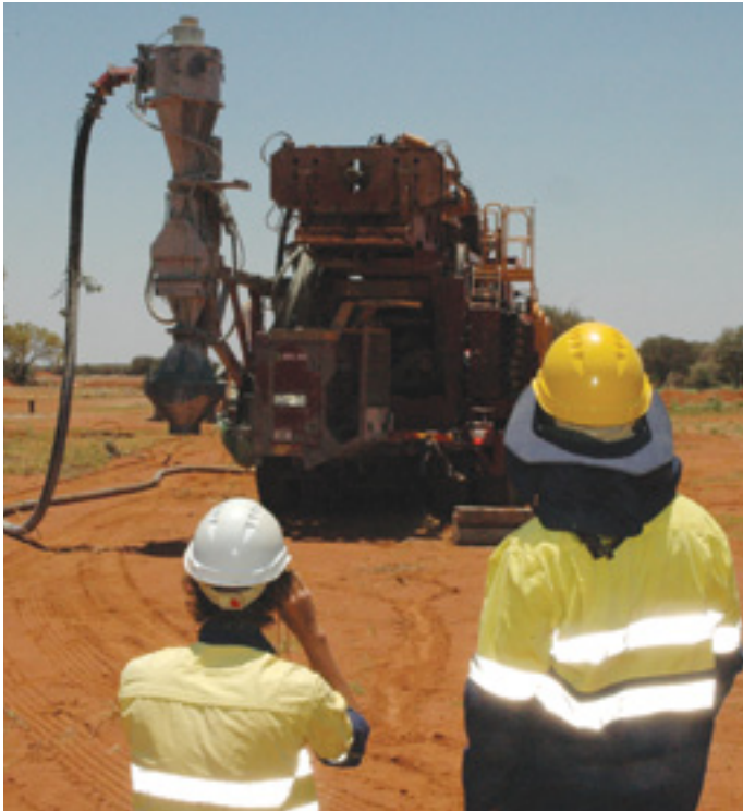
With the RC rigs testing for parallel structures to Wilber, getting the angle spot on is key for the Doray geologists
