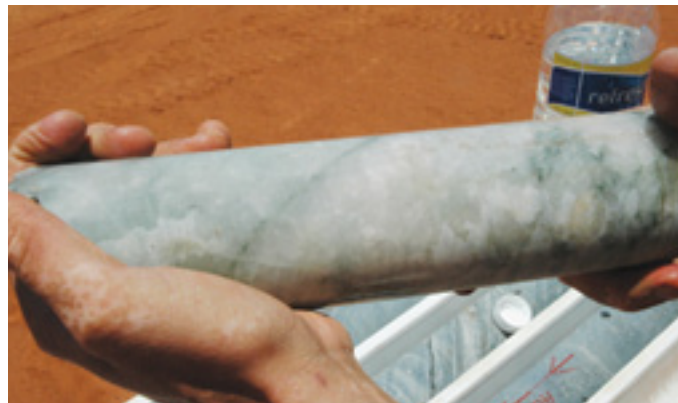
Abundant in pyrite, the high-grade gold is actually locked inside the green lines in the quartz vein
